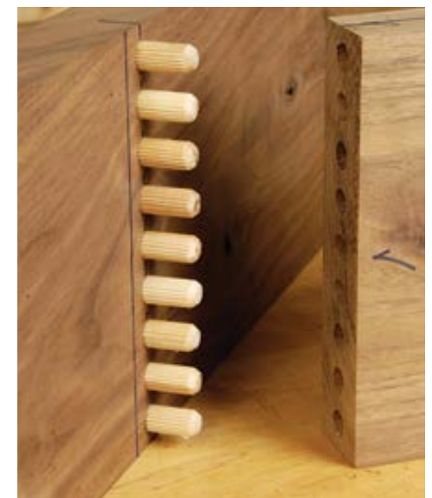
Using the index pin, a continuous row of perfectly aligned dowel holes is child's play
