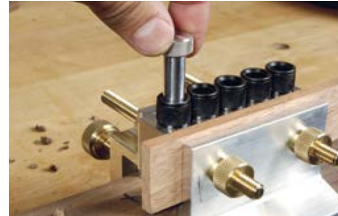
For edge jointing boards an index pin is used to create a line of evenly spaced dowel holes
