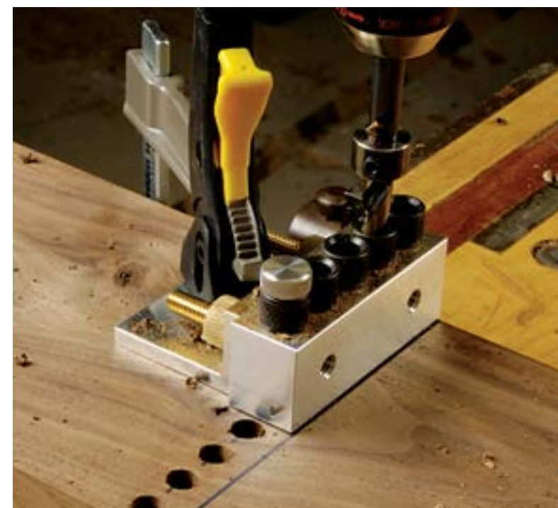
An offset line of 12mm from the centreline is required for face drilling
