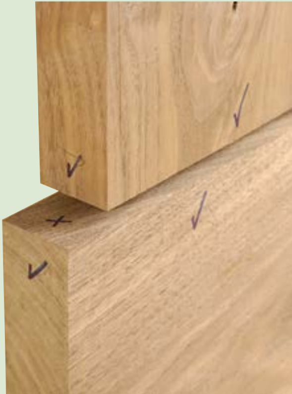
Place check marks on the facing edges of the mating components and a cross on the face or edge to be drilled
