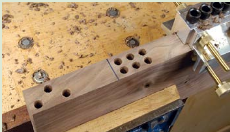
The drilling sequence can be adapted to suit the application
