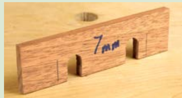
Make up some shims; these will enable you to work with the most common-sized stock in your workshop
